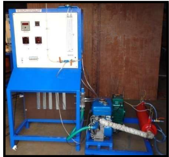
4 STROKE PETROL ENGINE TEST RIG WITH ELELCTRICAL LOADING
