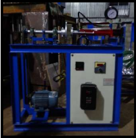
BREAK LINING FRICTION TEST RIG
