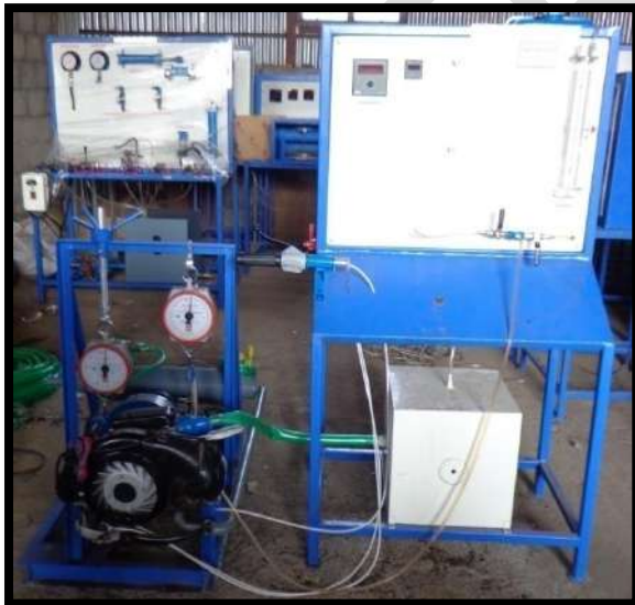
TWO STROKE PETROL ENGINE WITH ROPE BRAKE DYNAMOMETER
