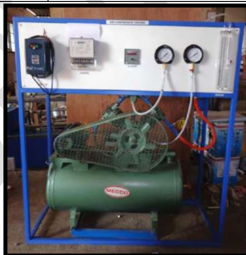
Two stage reciprocating air compressor test rig
