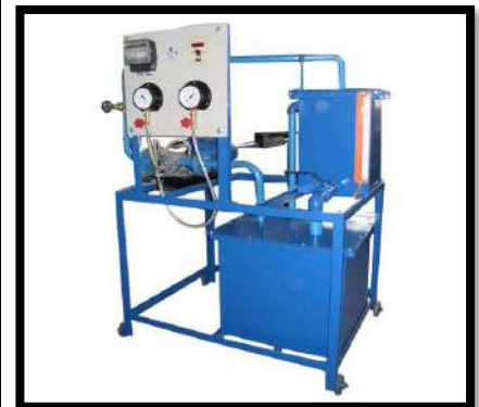
GEAR PUMP TEST RIG
