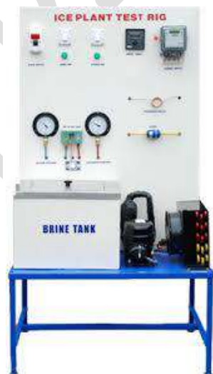
ICE PLANT TEST RIG
